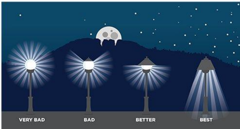
Light Fixture Shielding 184
